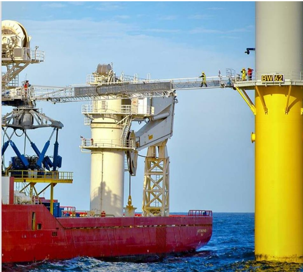
Figure 1: Walk-to-work arrangements for an offshore wind turbine service vessel.
